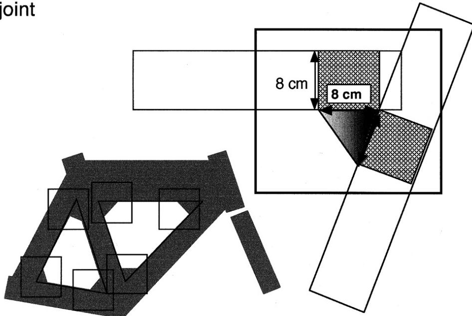
*The joint between frame section must fall within the highlighted triangle whose two sides have the same measurement as the height of the section, I.E. 8 cm.*
